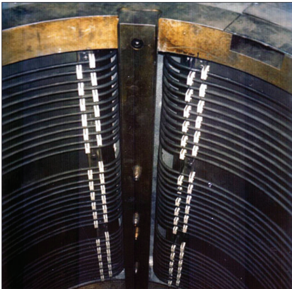
Figure 2b. Radiation heaters that are part of the container mantle heating system ready before installation.
