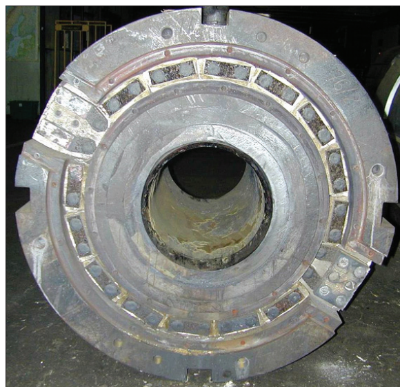
Figure 1. An example of a type of aluminum extrusion container with internal induction heating coils welded in place.
