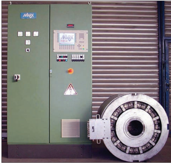
Figure 7. The brain that processes information and data and maintains linear control of radial and axial temperature distributions in the Smart Container.
